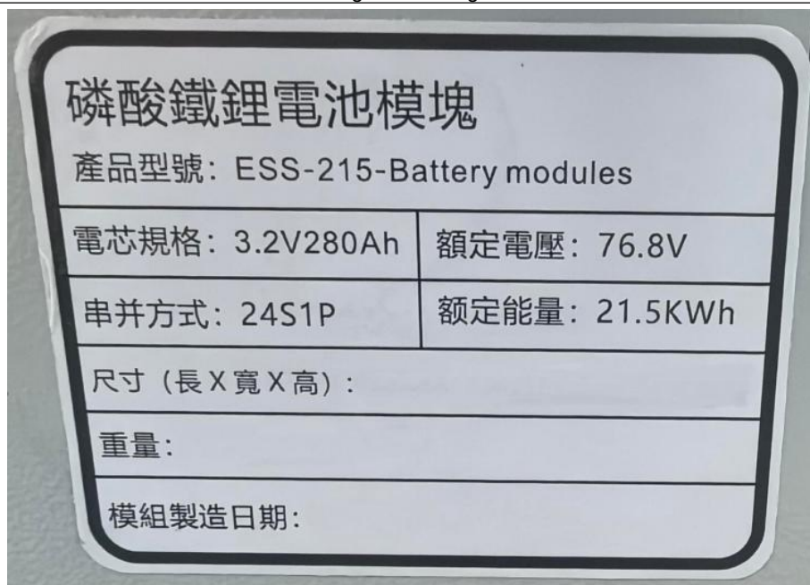
Photo 7 模組標籤特寫 Label close-up of module
