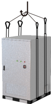
Figure 5.2.1-Lifting diagram of the 215 kWh air-cooled integrated energy storage cabinet (industrial/commercial).
